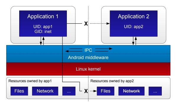
Figure 3.1: Each Android application is running in its own sandbox. Process isolation is enforced by the underlying Linux kernel which restricts the access to file system resources. IPC is possible through the Android middleware.
