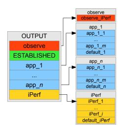
Figure 7.1: Firewall design for our test scenarios.
