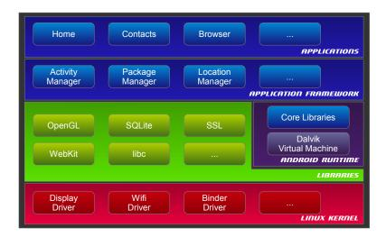
Figure 2.1: The system architecture of Android consists of five layers: A Linux kernel, several native libraries, the Android Runtime, an application framework and an application layer.
