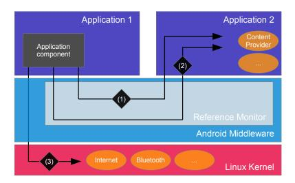
Figure 3.2: Permissions are enforced implicitly by the Android middleware (1), explicitly inside the application (2), or by the Linux kernel (3).
