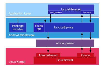
Figure 6.1: Interaction between the different modules. The left half illustrates firewall configuration, whereas the right half illustrates dynamic Internet requests.
