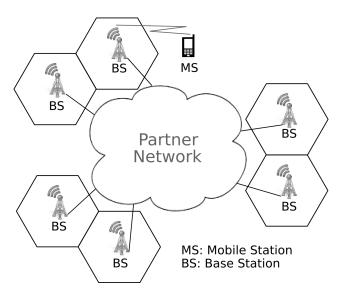
Figure 3.1: Mobile network architecture
