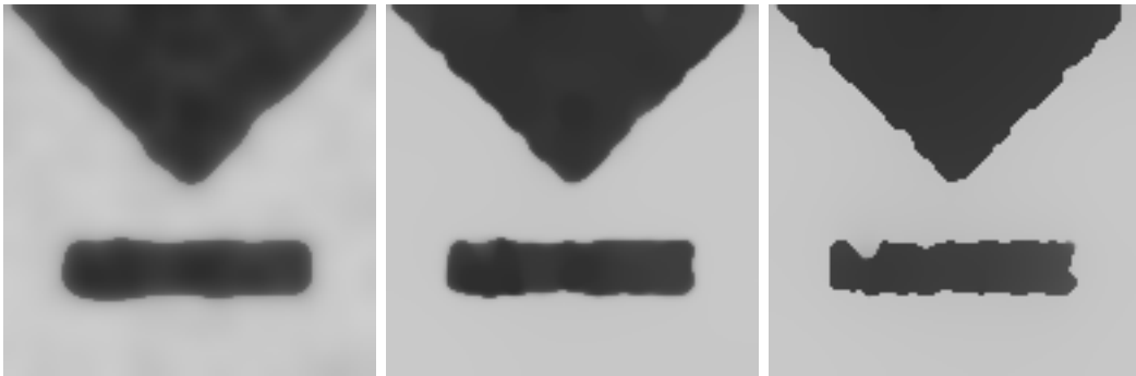
Figure 4.10: Noisy image filtered with moment preserving diffusion and different diffusivity functions g, p = 3, s = 127.5 ; Left: Linear diffusion, implicit scheme, \sigma = 0.1 , 100 iterations; Middle: Charbonnier diffusivity, AOS scheme, \tau = 5.0, \sigma = 0.0, \lambda = 0.05 , 100 iterations; Right: Perona-Malik diffusivity, AOS scheme, \tau = 5.0, \sigma = 0.0, \lambda = 0.12 , 100 iterations.
