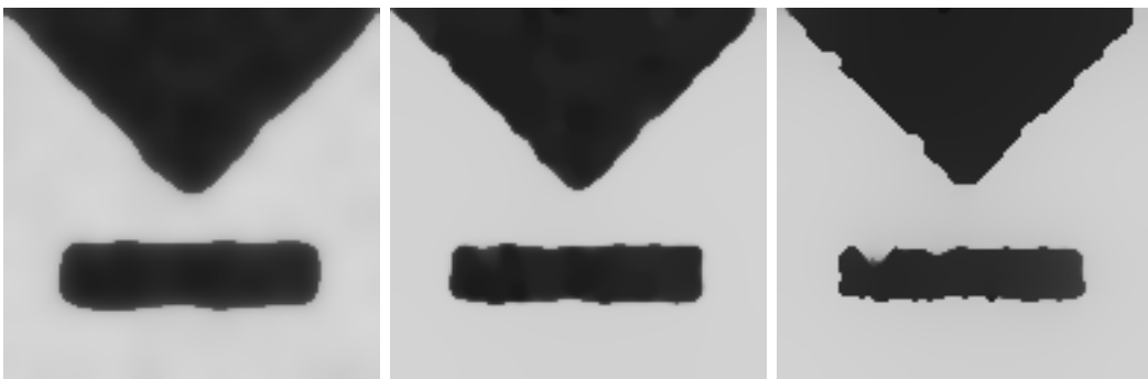
Figure 4.11: Noisy image filtered with moment preserving diffusion and different diffusivity functions g, p = 5, s = 127.5 ; Left: Linear diffusion, implicit scheme, \sigma = 0.1 , 100 iterations; Middle: Charbonnier diffusivity, AOS scheme, \tau = 5.0, \sigma = 0.0, \lambda = 0.12 , 100 iterations; Right: Perona-Malik diffusivity, AOS scheme, \tau = 5.0, \sigma = 0.0, \lambda = 0.21 , 100 iterations.
