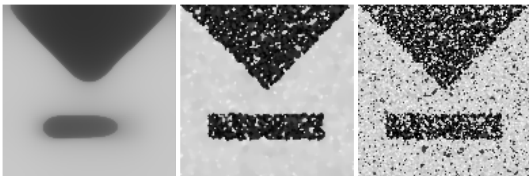
Figure 4.4: Influence of parameter p on the moment preserving diffusion, AOS scheme with Charbonnier diffusivity, s = 127.5, \tau = 5.0, \sigma = 0.0, \lambda = 0.1 , 50 iterations; Left: p = 3 ; Middle: p = 5 ; Right: p = 7 .
