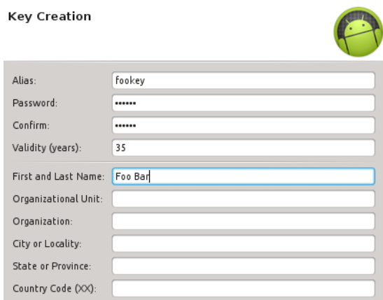
Figure 6: Create a new key. The filled fields in the figure are mandatory. Android requires, that the key must be valid at least 35 years.
