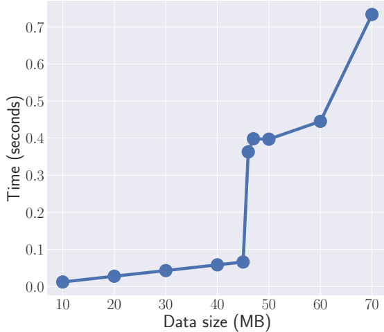
Figure 3: Overhead in seconds to load additional data for a defense mechanism preventing model stealing, namely Prada [17].
