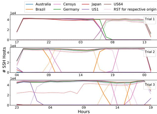
**Figure 12: Temporal Blocking by SSH hosts in Alibaba Networks**—Across all origins using only one source IP, Alibaba intermittently detects scanning and thus causes all SSH hosts to RST the connection after completing a TCP handshake.
