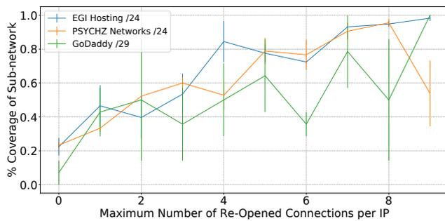
**Figure 13: Scanning Probabilistic Temporarily Blocking Hosts**—Increasing the number of times to retry a failed TCP connection increases the probability that a probabilistic temporarily blocking IP successfully completes an SSH handshake.
